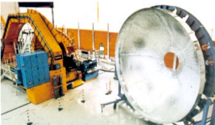
Ariane 5 tank bottom, shot peen formed, diameter 5.80m, sheet thickness 1.4-3.5 mm
